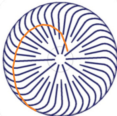
Ore exits at 1 o'clock using a vortex vane
