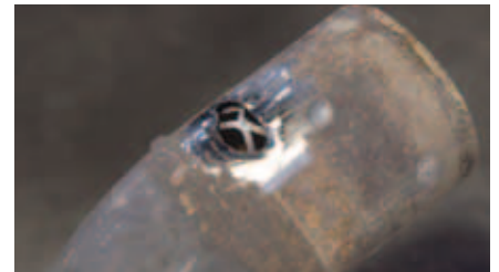
The wire mesh reinforces the repair area and forms a mechanical backing for the epoxy
