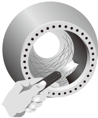
Figure 1. Epoxy putty is used to rebuild worn areas of volute
