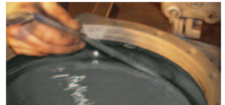
Coating a pump volute with LOCTITE® Nordbak Brushable Ceramic
