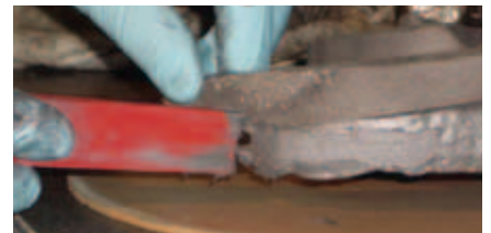
Repairing a pump impeller with LOCTITE® Fixmaster Wear Resistant Putty
