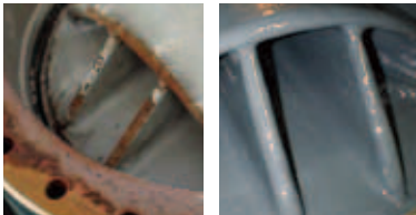
The corroded butterfly valve before and after repair
