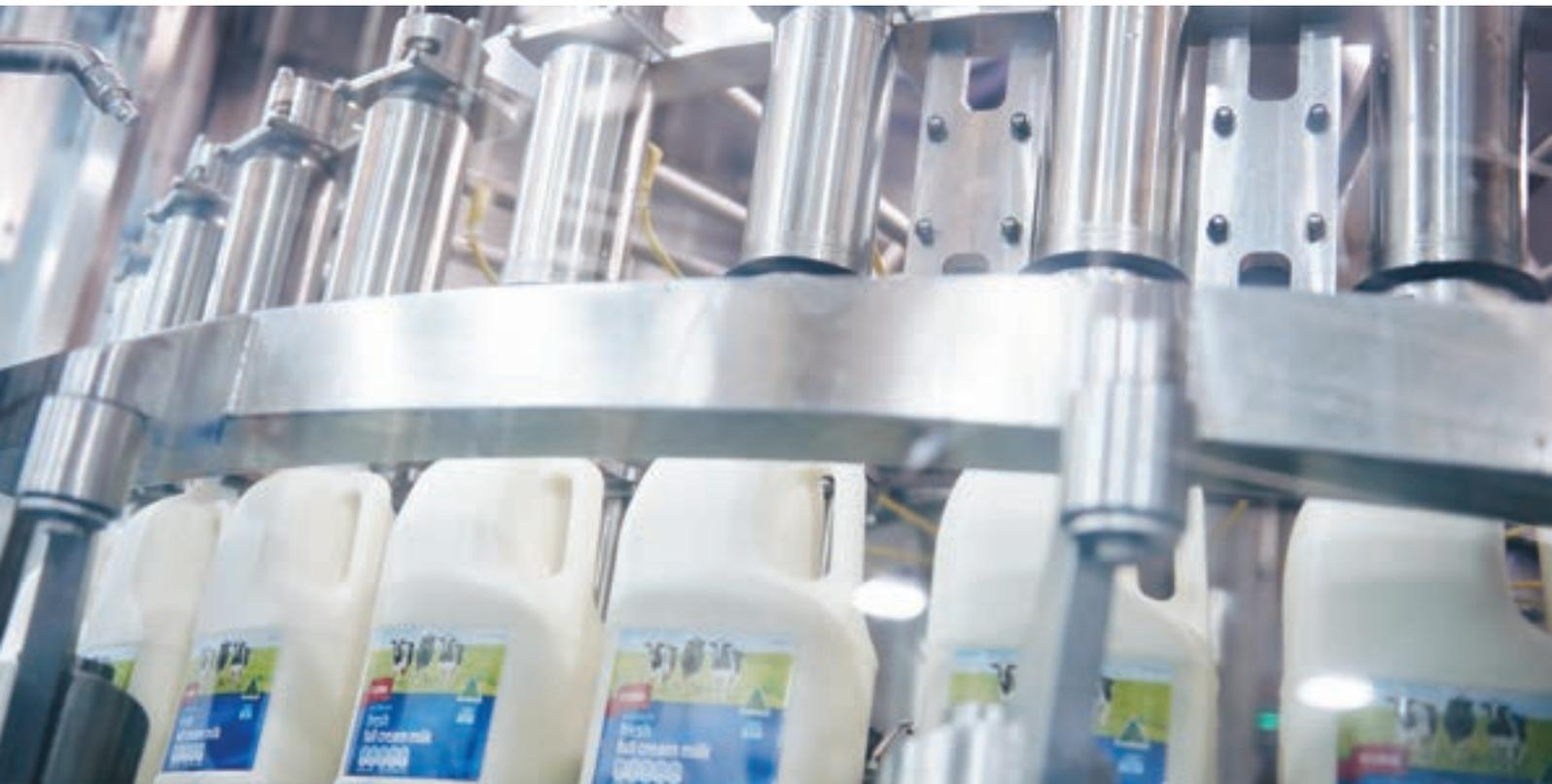
Our new Devondale Dairy Beverages Centres in Melbourne and Sydney were designed, built and commissioned in 18 months. The chilled milk facilities are world-class, featuring complete end-to-end automation, utilising the latest milk processing and filling technology to operate at high speeds with energy efficiency. Each plant is capable of processing 50,000 litres of milk per hour and producing 150 million litres of chilled milk per year.
